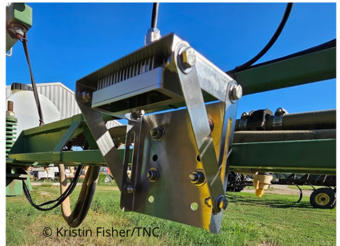
Image: PlantMap3D Camera mounted to spray rig for mapping
